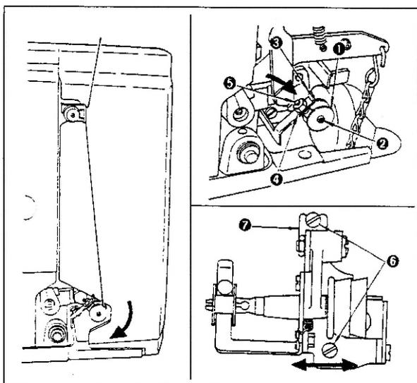
1. Attach bobbin ❶ to bobbin winder spindle ❷.
