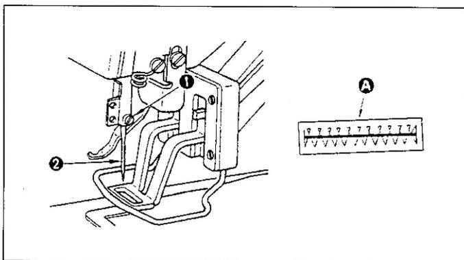
Loosening setscrew ❶, insert needle ❷ fully into the needle bar hole with the long groove of the needle facing towards you, then tighten setscrew ❶.
