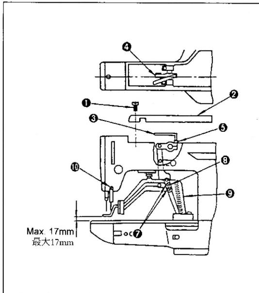
The lift of the work clamp foot can be adjusted up to 17mm
