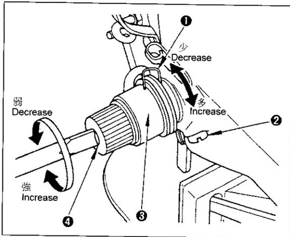
The normal stroke of thread take-up spring ❶ is 6 to 8 mm, and the tension at the starting point is 0.3 to 0.5N.
