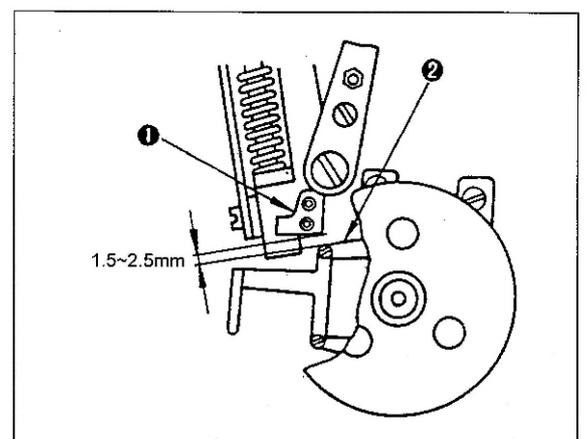
1. Loosening two setscrews ③, perform adjustment so that a 0.2 to 0.5mm lateral clearance is provided between safety plate ① and lifting lever ② when the work clamp foot is up at the time of stop motion, and a 1.5 to 2.5mm longitudinal clearance between them when the work clamp foot is down.
