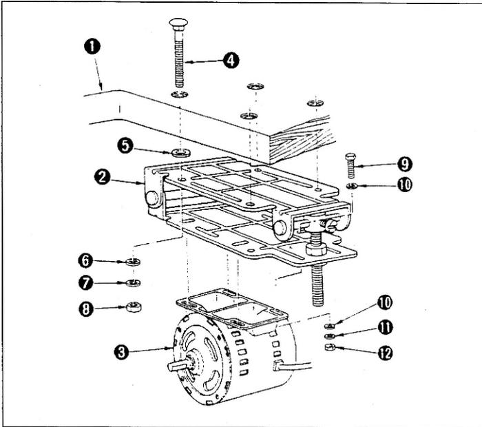
1. Attach motor base ② to table ① using bolt ④, vibration-proof rubber pad ⑤, washer ⑥, spring washer ⑦, and nut ⑧.
