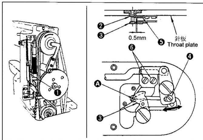
1. Remove starting lever tension spring ❶, and start the machine. (The work clamp foot stays down when the machine stops.)
