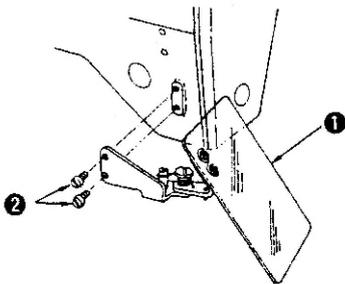
5. Be sure to fix eye protecting cover ① with screw ② on machine frame before putting the machine into service.
