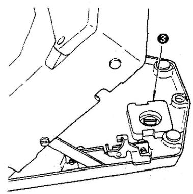
4. Before starting a machine which has been newly set up or has not been used for a long period of time, apply a few drops of the lubricating oil to main shaft components through hole ①, one drop to the racing surface ② of the shuttle race, and infiltrate amount of the lubricating oil to the machine bed oil felt ③.
