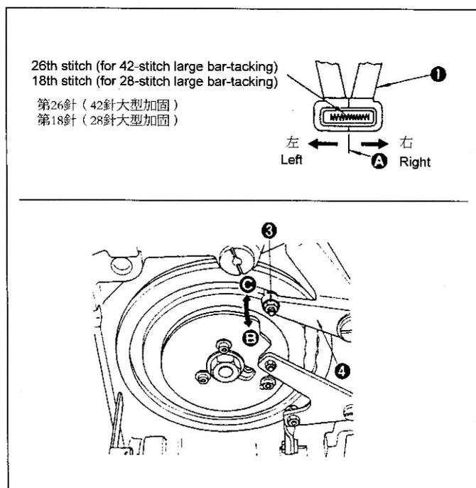
Loosen nut ❸, and move feed across regulator in direction ❷ to shift lateral ❹ center of work clamp foot ❶ to the right or in direction ❸ to shift it to the left.
