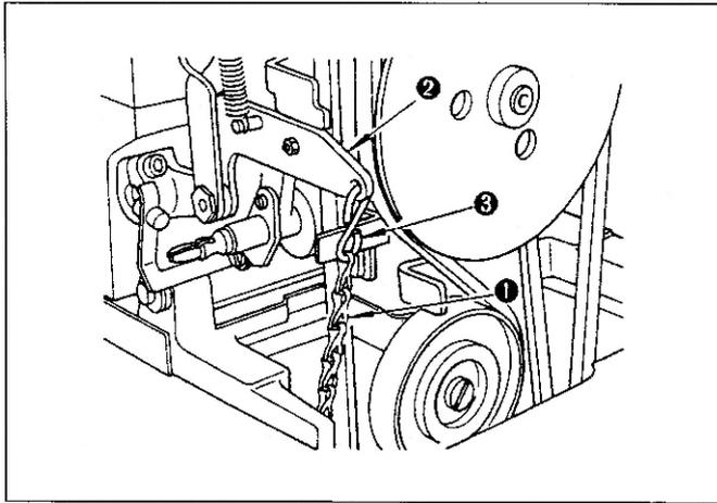
Hook S-shaped hook ③ into the hole in the tip of starting lever ②, and attach chain ① to the S-shaped hook.
