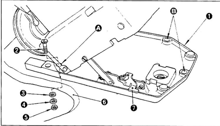
1. Install bed mounting base ① to machine table ⑥ using bolts ②, flat washers ③ and ④, and nuts ⑤ (each 3 pcs.).
