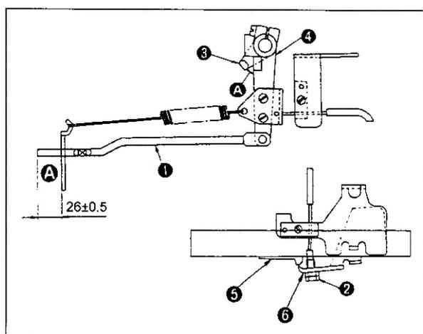
1. Confirm that the pawl section of thread release lever ⑥ rides completely the mound section of disk floating notch ⑤ when the machine is in the stop-motion state. At that time, adjust with nut ② of the wire setting screw so that the protruding amount of tension release bar ① becomes  $26 \pm 0.5$ , and tighten it.
