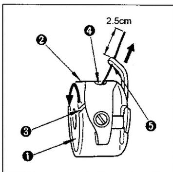
1. Hold bobbin ❶ in hand so that it spins counterclockwise and set it in bobbin case ❷.
