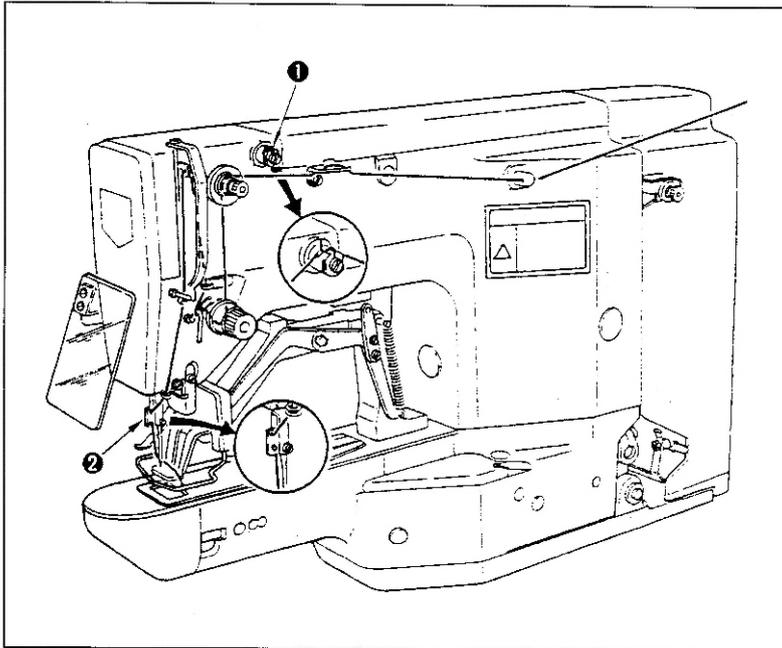
Thread the machine in the order as shown above. Leave thread of approx. 4cm on the needle.
