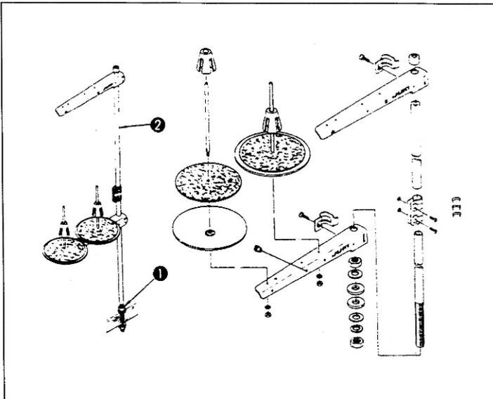
Assemble the thread stand, and set it in the hole in the table.
