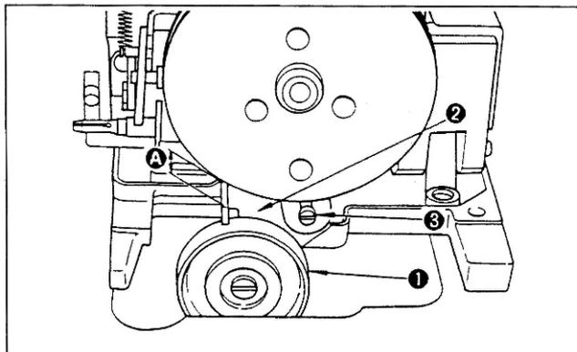
Fix idler pulley ① to mounting plate ② by setscrew ③.
