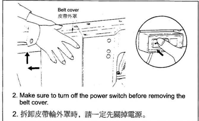
2. Make sure to turn off the power switch before removing the belt cover.
