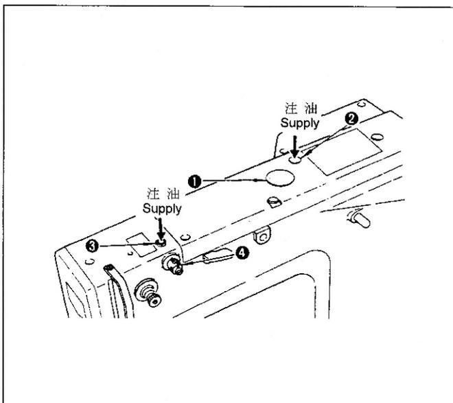
1. Lubricate the machine once a day from lubrication hole ②. The machine can also be lubricated by removing rubber plug ①.
