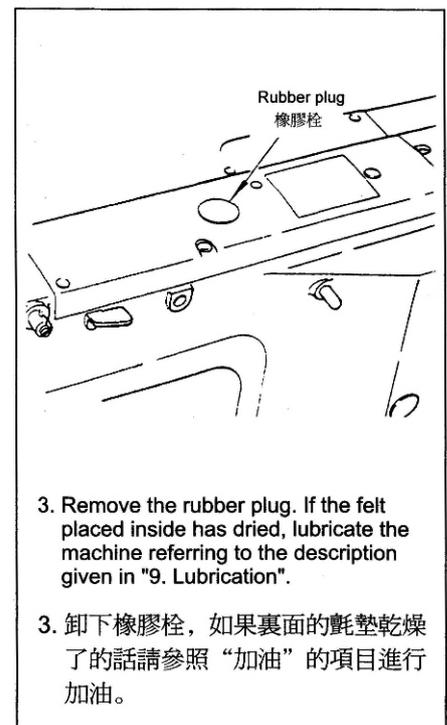
3. Remove the rubber plug. If the felt placed inside has dried, lubricate the machine referring to the description given in "9. Lubrication".
