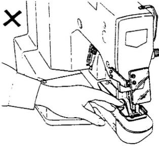
1. Do not place your fingers near the work clamp foot while the machine is in operation.
