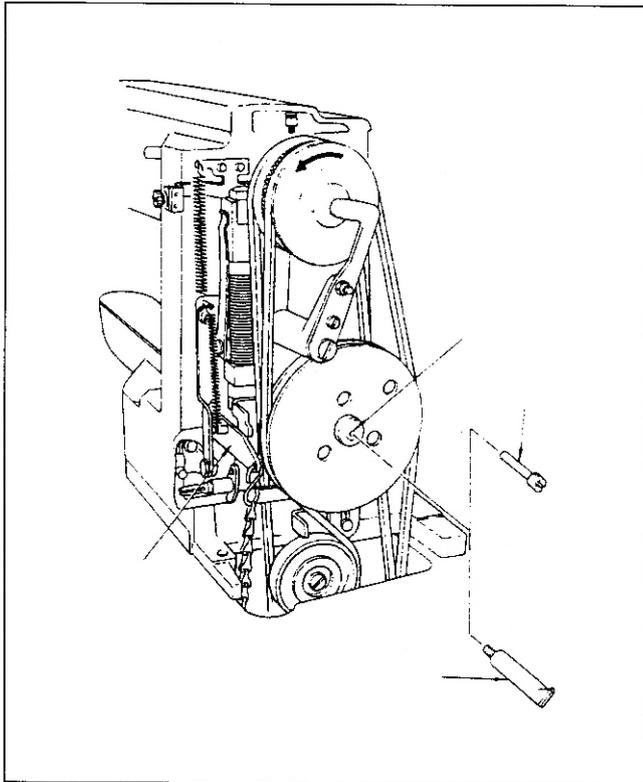
{ Supply grease to the reducer in accordance with the following procedure when the machine has been used for more than half year or if it chatters. }
