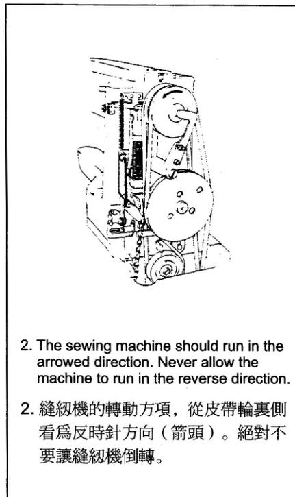
2. The sewing machine should run in the arrowed direction. Never allow the machine to run in the reverse direction.
