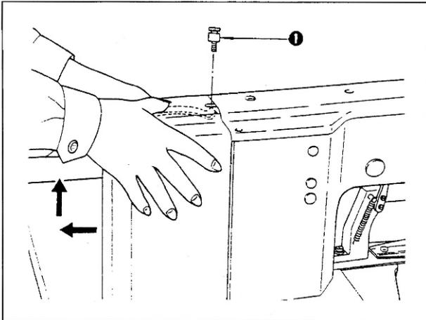
To remove the belt cover, loosen screw ❶ and tilt the belt cover away from you until it comes off then lift it.
